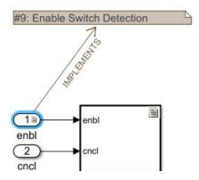
The annotation displays the ID, the summary, and the relationship between the block and the requirement. In this example, the block implements the requirement. For other possible relationships, see "Requirement Links" on page 2-6.
