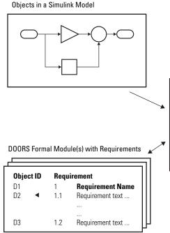
Enter requirements in the DOORS formal module and link them to objects in the DOORS surrogate module, so you can navigate from requirements to Simulink objects.
